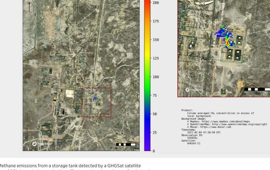
Photo: Methane emissions from a storage tank detected by a GHGSat satellite in February 2021. An emissions reduction effort was already underway for the tank.
