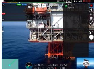
**Photos:** Drone pilots using laser and OGI technology to conduct a methane emissions inspection of a Chevron platform in the Gulf of Mexico.
