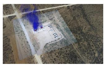
**Photo:** Methane emissions detected in June 2021 using Bridger Photonics aerial lidar technology at a remote centralized production facility tank battery in the Permian Basin. Color added for effect. An October 2021 follow-up flyover detected no emissions after facility repairs were made.
